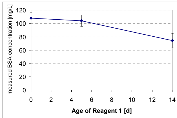
Figure 44: Stability of reagent 1 measured with BSA 100 mg/L and SIA method (error bars: SD, n=5)
