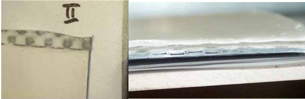
Figure 42 – Pictures of the surface and section of the nanoweb coated membrane sealed to the support with the A3 procedure. No differences were found on the membrane treated with fluorocarbon.
