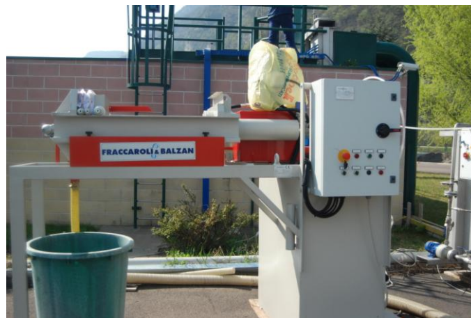
Figure 2: Pilot-scale filter press for dewatering tests
