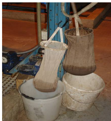
Figure 7 Sludge supernatant preparation
