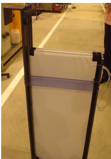
Figure 8 Flat sheet membranes immersed in the pilot plant
