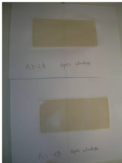
Membranes after fouling Figure 20 Membrane samples after fouling
