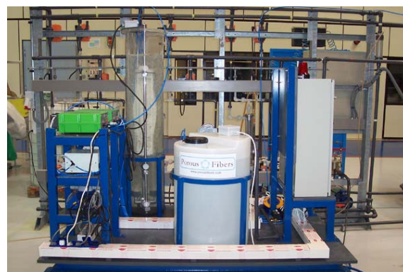
Figure 2. Pilot plant of the submerged membrane bioreactor (SMBR) for wastewater treatment.
