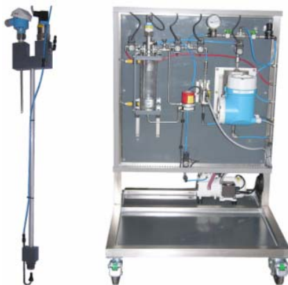
Figure 1: The MBR-VFM set-up: (left) fouling sensor, (right) measuring apparatus
