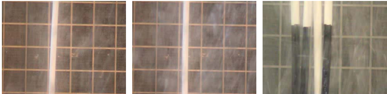
Aeration = 4 (left) resp. 6 (centre) L/min. Right: Bundle with 4 fibres, aeration = 6 L/min.
