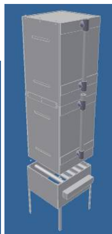
Double deck 140 m 2 Air flow rate 0,2 – 0,35 Nm 3 /(h*m 2 )
