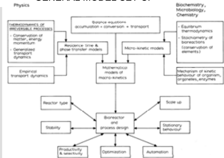
Fig. 1.2. The structure of (biochemical) reaction engineering. (From Roels, J.A. (1982) J. Appl. Chem. Biotechnol. 32, 59.)
