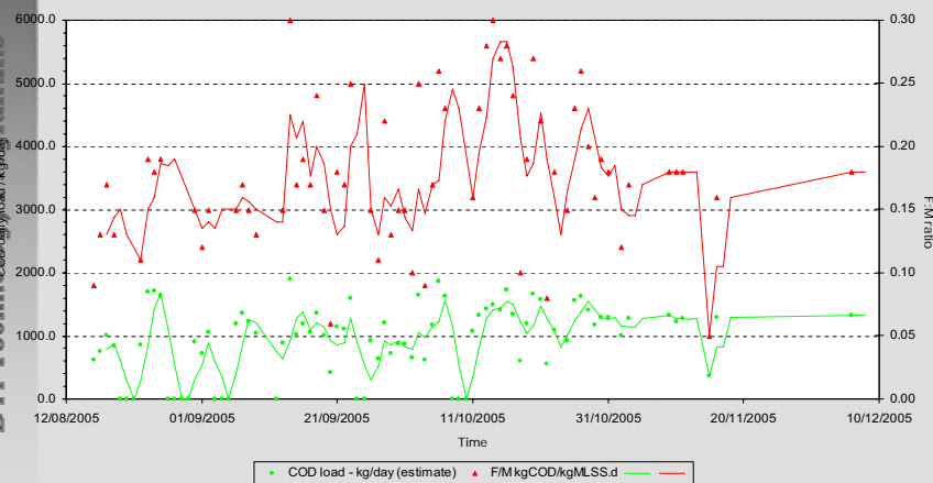
Ledbury AMBR - COD removal
