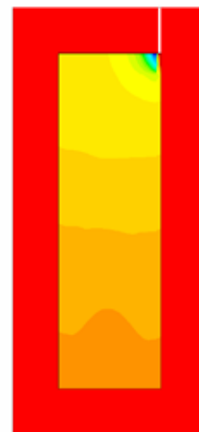
Figure 14 Pressure distribution [N/m 2 ]; scaled from -77000.0 [blue] – -74000.0 [red]
