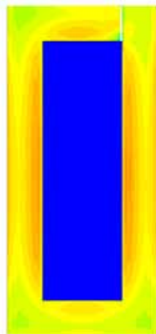
Figure 13 Pressure distribution [N/m 2 ]; scaled from -0.01 [blue] – 0.01 [red]
